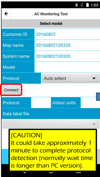
Select correct protocol, then tap Connect to detect protocol For Altherma hydro, always select Altherma (auto select does not work in this case)
